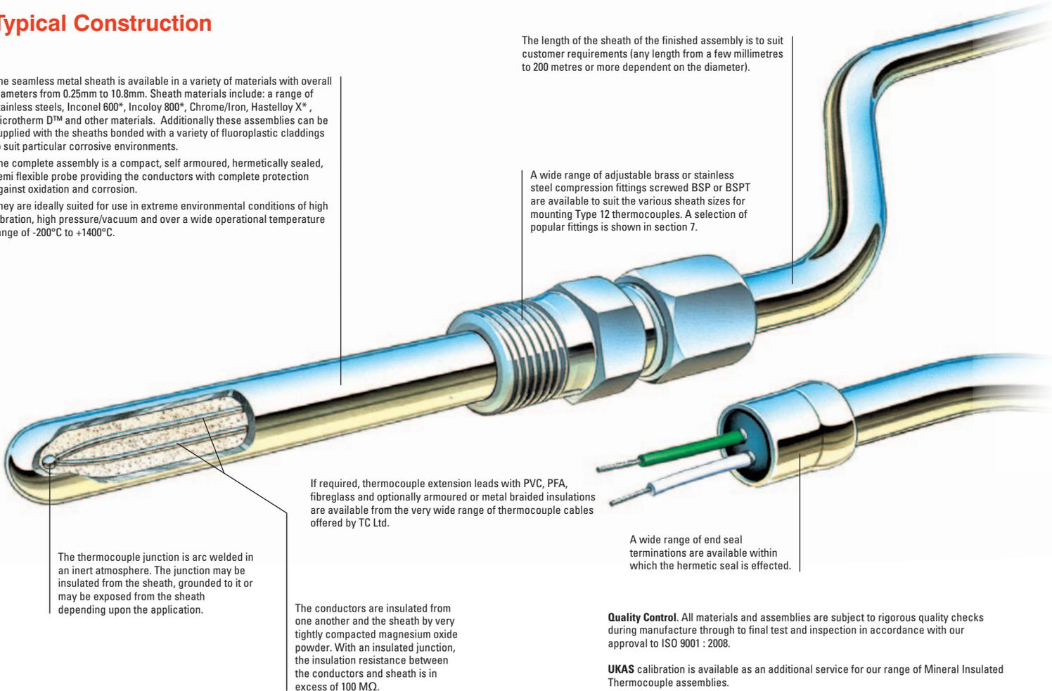
The thermocouple junction is arc welded in an inert atmosphere. The junction may be insulated from the sheath, grounded to it or may be exposed from the sheath depending upon the application.
