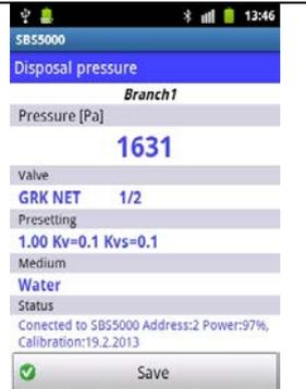
6. Measuring of Initial flow in branch. SBS 5000 Standard will automatically choose the correct valve and presetting according to the branch selected. The Initial flow measured will be saved along with the rest of the branch data.
