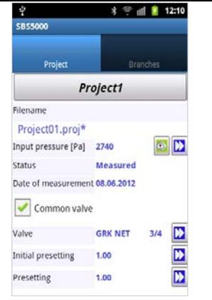
5. You can measure Input pressure using the Measure icon in its line. The calculated Common valve presetting can be viewed in the Presetting Window at the end of project balancing.
