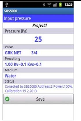
4. Connect SBS 5000 Standard measuring unit to the balancing valve at any branch and select the appropriate branch in the Branch tab. It is necessary to measure both the Flow through the valve with Initial presetting of the balancing valve and the Disposal pressure in the branch with the balancing valve being closed. The value measured will be automatically filled in the corresponding field.
