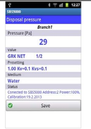
5. Measuring of disposal pressure. Close the balancing valve in the branch prior to measuring the available pressure in the branch. The value measured will again be saved along with branch data.
