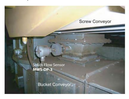
This is an actual application of the Solids Flow Sensor using the filter function.
