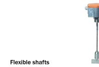
The flexible shaft consists of an 8 or 12 mm rugged steel cable. The advantage of a flexible shaft: There is no continuous bending via lateral stress through movement in the bulk product or when the bulk material hits the steel cord and the paddle wheel. If the silo is empty, the steel cord is tightened with a tightening weight.
