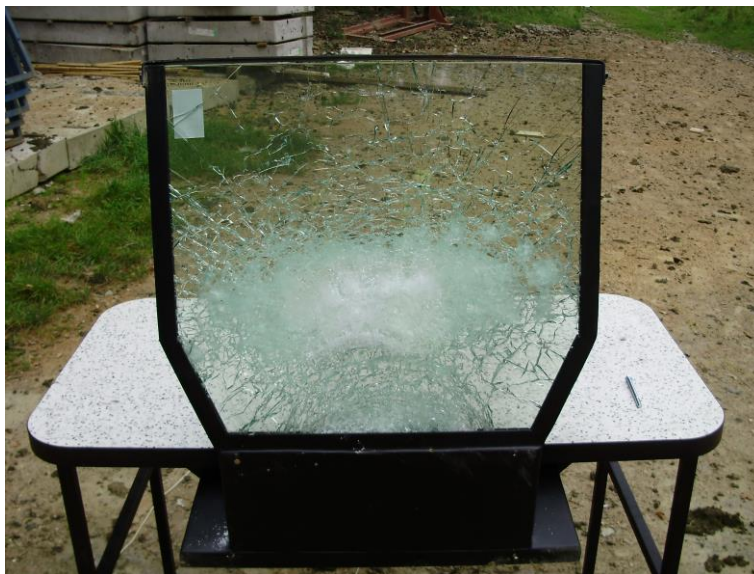
The ballistic proof glass after explosion of 10 g PBX (Semtex 1A) in steel tube, 10 cm from the glass.
