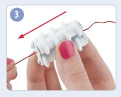
Fold the rollers closed tightly, then pull the wire through to straighten.
