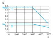
M: Torque in Nmn: Speed in rpm1: Peak torque2: Continuous torque
