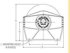
Dimensions E and F are based on the Standard Motor. Length will vary with optional motors.
