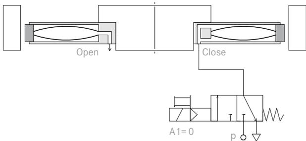
RotoClamp standard outer clamping active
