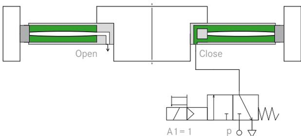
**Release RotoClamp Outside** The spring diaphragm is bent on assembly and the distance between the two radial contact surfaces at the inner and outer diameter of the spring is reduced. The clamping element is opened in this state.
