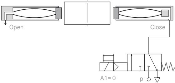
RotoClamp standard inner clamping active
