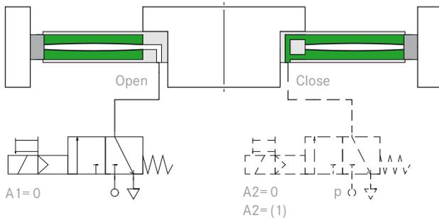
**Release RotoClamp Outside** Adding pressurized air to the inner spring diaphragm chamber (open, 4 or 6 Bar) and venting the outer spring diaphragm chamber (close) bends the diaphragm and the distance between the two radial contact surfaces at the inner and outer diameter of the spring is shortened. The clamping element is opened in this state.
