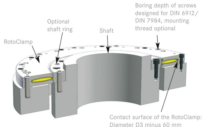
Make sure that there is a rigid connection and correct attachment to transmit the forces!
