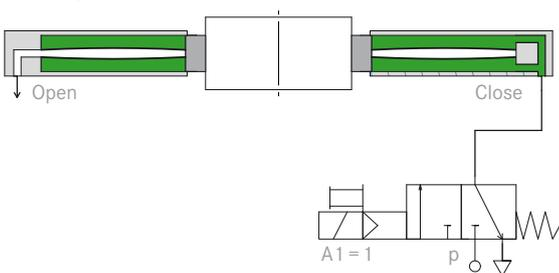
**Release RotoClamp Inside** Adding pressurized air to the inner spring diaphragm chamber (open, 4 or 6 Bar) and venting the outer spring diaphragm chamber (close) bends the diaphragm and the distance between the two radial contact surfaces at the inner and outer diameter of the spring is shortened: The clamping element is opened in this state.
