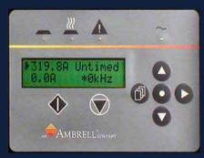
EASYHEAT features a front panel programmable controller allowing you to define up to four different heating profiles, each with up to five time/power steps.
