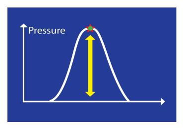
Commonly, a mounted offset blanket is monitored by measuring the height of the blanket in millimeters or inches. Compared to the precision of the **Pressure Indicator**<sup>TM</sup>, however, this is something of a "trial and error" approach to estimating the pressure level between plate and blanket, and blanket and impression cylinder.
