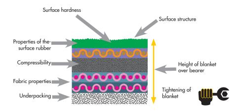
The above illustration shows the multiple blanket properties that combine to determine nip pressure. Blanket properties can vary over time. For example, through usage, the compressibility layer will "sink", reducing nip pressure. At the same time, the surface rubber hardens, producing an increase in nip pressure.
