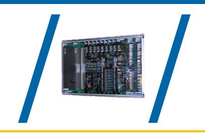
The ACE 100 System Node components comprise mainly of the Input Card, Output Card, Supervisory Card, Sound Palette and Power Supply Card.
