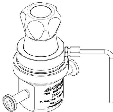
Optional 1/8" captured vent and/or leakage connection.
