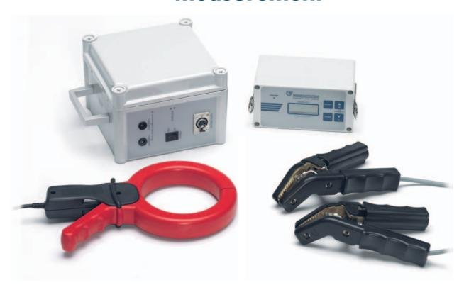
NCM-20 has two voltage clips by which the test current is supplied into the bank. The voltage output is short-circuit proof.
