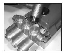
5. Tap the back of the valve casing (29) with a rubber mallet.
