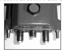
13. Replace copper ring (24E) onto plunger bolt (24B). Slide plunger bolt assembly (24) into ceramic plunger (24A). Apply a light film of loc-tite to plunger bolt threads and place plunger assembly onto stainless steel plunger base (22) and tighten to 310 in.-lbs. (35 Nm) for SP100W(HK)/SP200W and 265 in.-lbs. (30 Nm) for SP351W.
