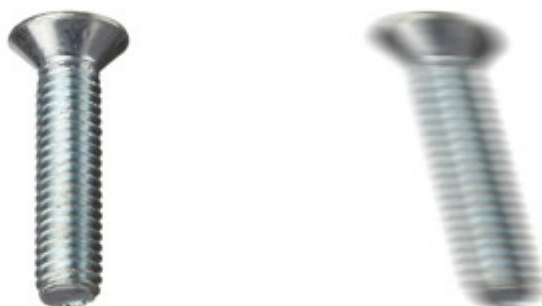
figure 4-5, rolling shutter mode, image of a horizontally moved object, long exposure time
