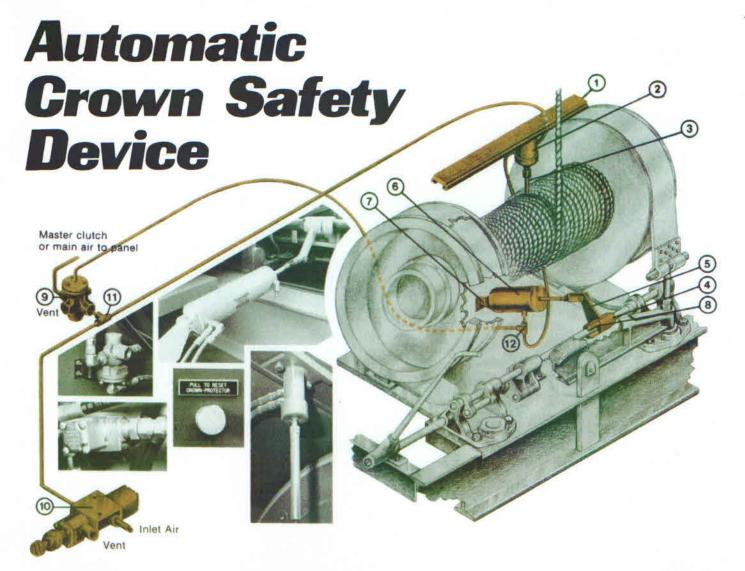
The Automatic Crown Safety Device is a safety aid installed on a drawworks drum to control the distance a traveling block may be pulled into the derrick thus eliminating the possibility of pulling the traveling block into the crown.
