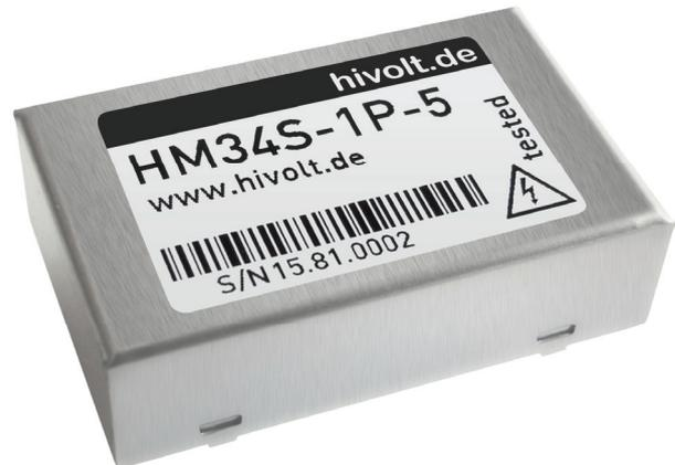
The HM34S Series is a family of high performance high voltage DC to DC converters. The converters' outputs feature protection against electric shock according to EN 61010-1:2010 / IEC 61010-1:2010-06 Edition 3.0 when connected to accessible parts. The short circuit output current is being limited to < 2mA under normal condition and < 15mA under single fault condition. The stored charge is < 45µC.
