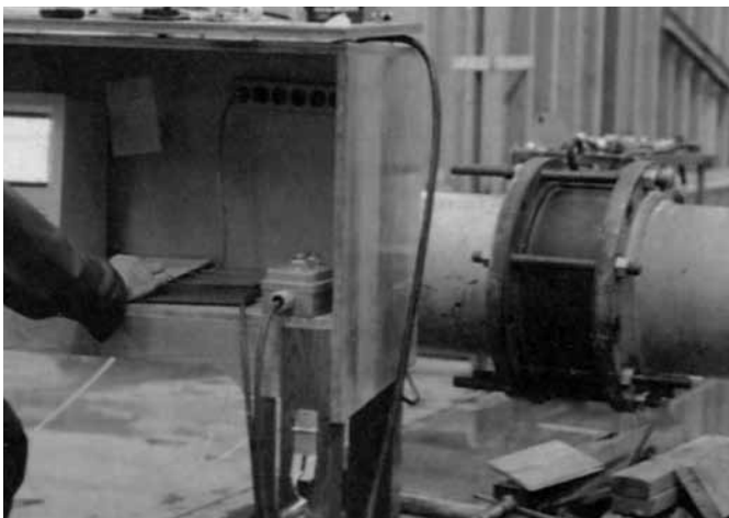
Actual flow testing for head loss characteristics. 1991, Conducted at Utah State University Water Research Laboratory, Logan, Utah
