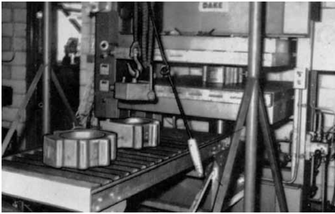
DDCV seals are compression molded under strict quality control standards. Every seal is tested.
