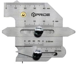
The gauge consists of main scale, height gauge, undercut depth gauge and multiple-purpose gauge and is specially used for the measurement of the bevel angle, height, width, gap and undercut depth of weldment, suitable for the detection of boilers, bridges, ships, pressure vessels and oil pipes.
