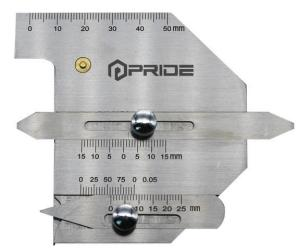
The gauge consists of main scale, height gauge, undercut depth gauge and multiple-purpose gauge and is specially used for the measurement of the bevel angle, height, width, gap and undercut depth of weldment, suitable for the detection of boilers, bridges, ships, pressure vessels and oil pipes.
