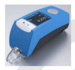
The right surface roughness on a gravure cylinder is not only decisive for a long lifetime of the cylinder but also for a smooth printing performance. Thanks to the Rz-Star measurement device you can now check your roughness in a matter of seconds. Additionally you can print out the measured values with the optional Bluetooth printer as evidence of your high quality standards.
