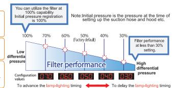
**WARNING**: The timing of the light can be set at five different levels.
