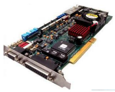
Turn your PC into an effective PCB fault finding system by incorporating the FaultFinder PCI card
