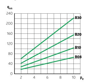
$p_e$  = overpressure [bar]  $q_{vn}$  = air consumption [m<sup>3</sup>/h]
