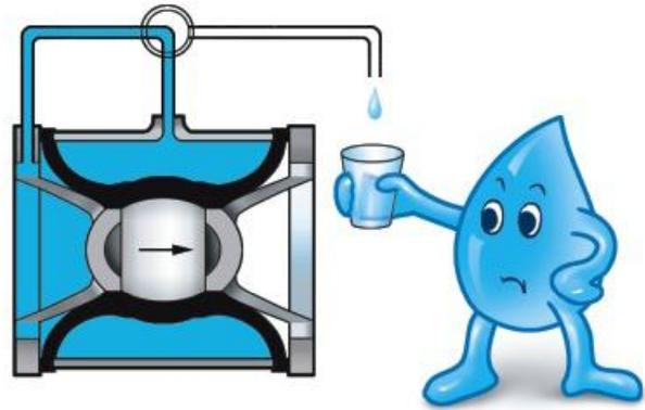
The **Inbal** Valve closes tightly when the pressure port is interconnected with the common port. The vent port is isolated.
