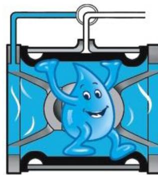
The **Inbal** Valve opens wide when the operating pressure is relieved from the control chamber. A minimum line pressure is required to hold the **Inbal** Valve in a fully open position. The flow through the valve is streamlined with low pressure loss.
